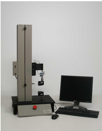
Model MT-1516 Universal Tester with Small Pneumatic Sample Grips and MT-2500 Quality Control Software
